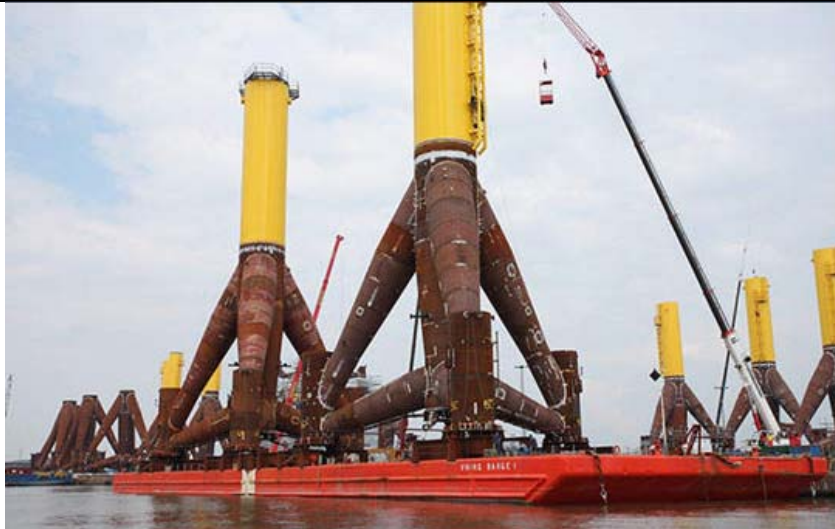
Figure 8: Wind farm components (tripod foundations) on a barge, considerably increasing windage of the vessel
